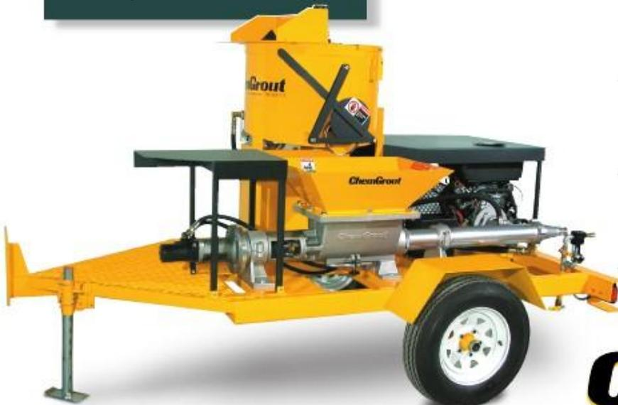
Powerful size 6 progressive cavity pump provides a smooth, easy to control delivery of both thick and thin materials.
